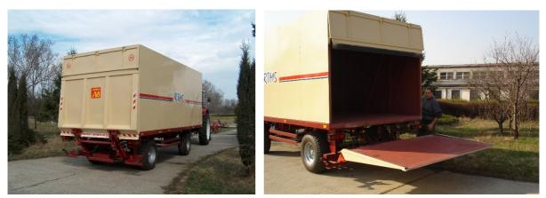
Fig. 1. Trailer with mobile shutter for transporting packed or containerised products made at INMA Bucharest – RTM5 [4]
