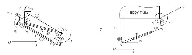
Fig. 7.**Defining position kinematic parameters of** mechanism (lifting phase)
