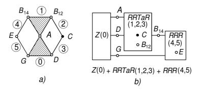
Fig. 5. Structural scheme of mechanism in Figure 4 (a); multipolar scheme and structural relation of the same mechanism (b)
