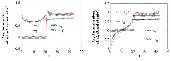
Fig. 9. Diagrams of angular velocities of mechanism elements
