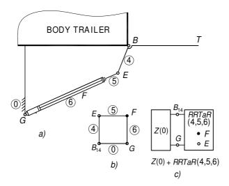
Fig.6. Mechanism of lifting shutter at the beginning of folding phase: a – kinematic scheme of mechanism; b – structural scheme; c – multipolar scheme and structural relation
